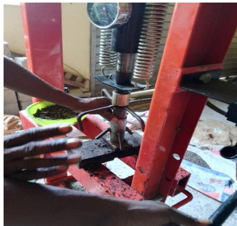
Plate 6: The Briquette Machine: Process of Pressing and Printing
