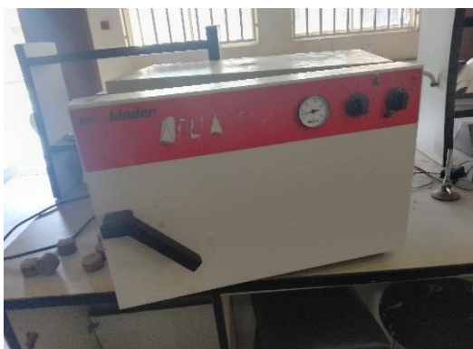
Plate 7: During drying process of the briquette
