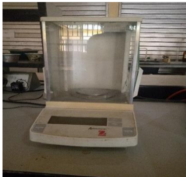
Plate 3: laboratory-type digital balance with 0.01-g precision
